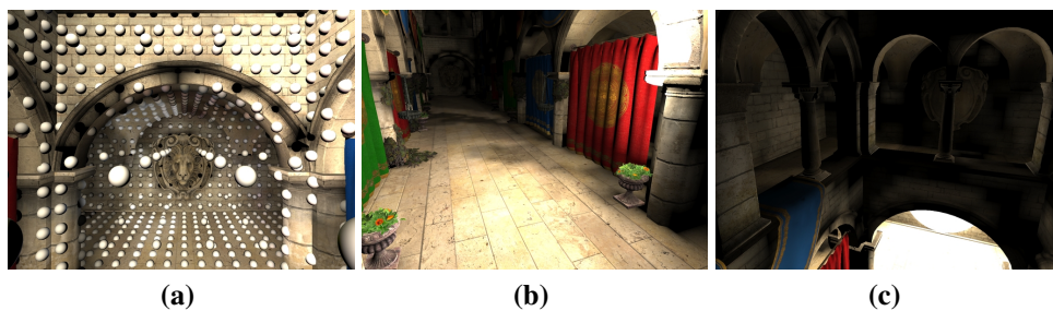
Figure 9. Possible artifacts of the algorithm. (a) Light map caches (black ones) are placed behind other geometry. This can be fixed by enabling backface culling during cache precomputation; (b) A small spotlight (top right) reveals discontinuities in linkage on the floor; (c) Single bounce light bleeding (amplified by \times 4096 ): the upper corridor should be black. The cause is that the hierarchy can merge clusters which cannot see each other.
